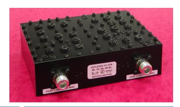
Microlab Model BK-71N is a Diplexer which allows combination and separation of the signals in the LTE band 698 - 793 MHz and the 824 - 894 cellular band. To minimize band inter-reaction, the inputs are well isolated and have minimal insertion loss over their respective frequency bands.
